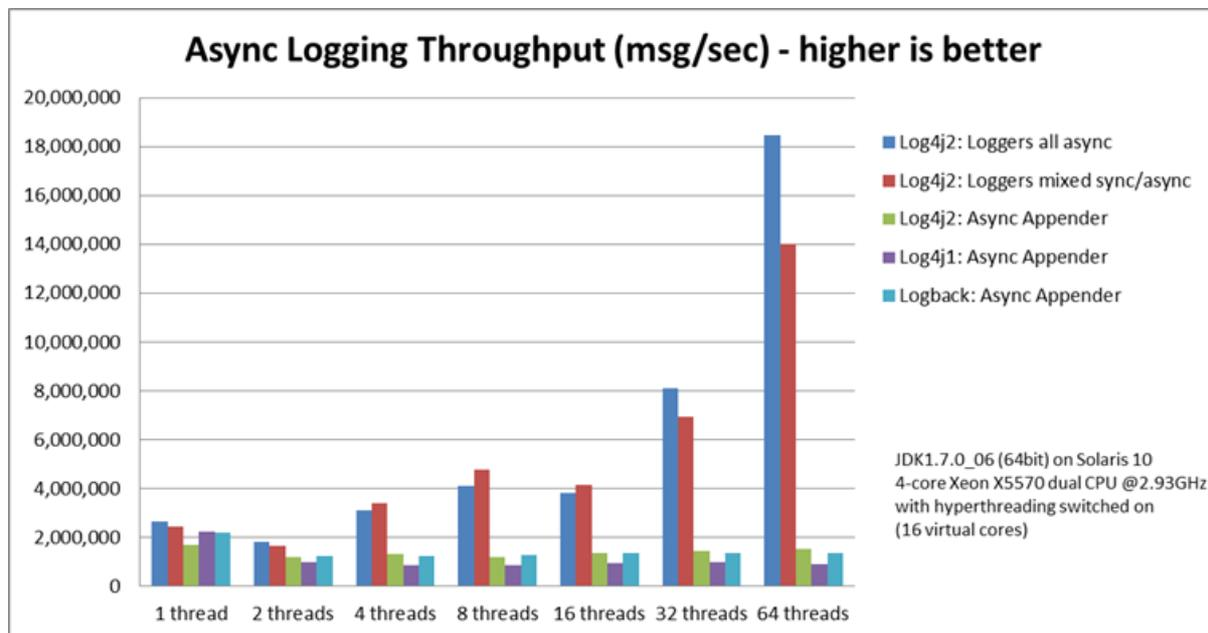
On Solaris 10 (64bit) with JDK1.7.0\_06, 4-core Xeon X5570 dual CPU @2.93Ghz with hyperthreading switched on (16 virtual cores):
