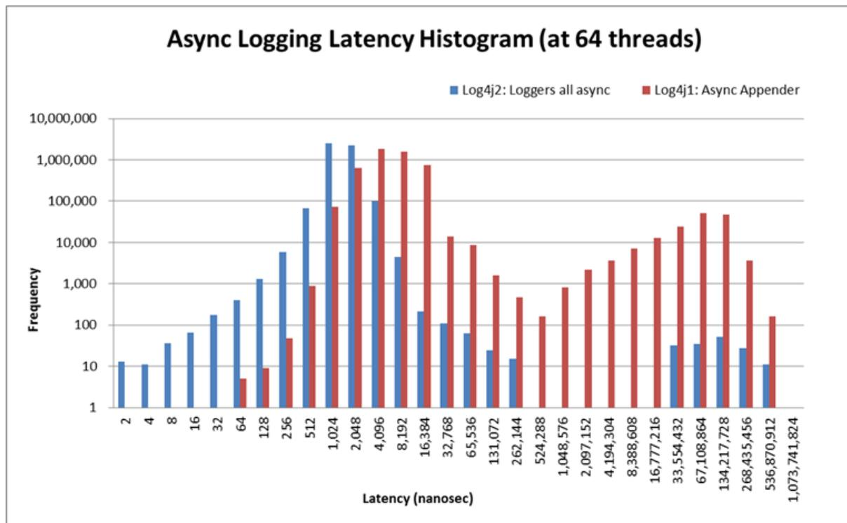
Note that this is log-scale, not linear. The above graph compares the latency distributions of an asynchronous logger and a Log4j 1.2.17 Async Appender. This shows the latency of one thread during a test where 64 threads are logging in parallel. The test was run once for the async logger and once for the async appender.
